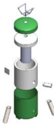
Figure 2: Views of the Designed Charcoal Fired Crucible Furnace a. side view b. isometric view c. top view.
